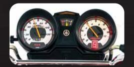
An easy-to-read speedometer with **GEAR INDICATION, FUEL GAUGE** and **TRIP METER.**
