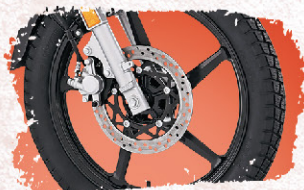
LONG SHOCK ABSORBERS WITH RUBBER BOOTS
